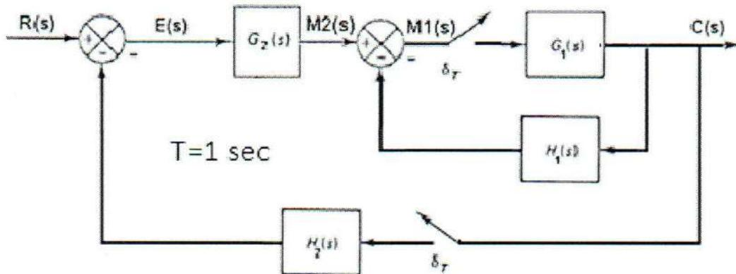
$$\text{Where } R(s) = \frac{1}{s}, \quad G_1(s) = \frac{K}{s+1}, \quad G_2(s) = \frac{s}{s+1}, \quad H_1(s) = \frac{5s}{s+1}, \quad H_2(s) = \frac{K}{s}$$
